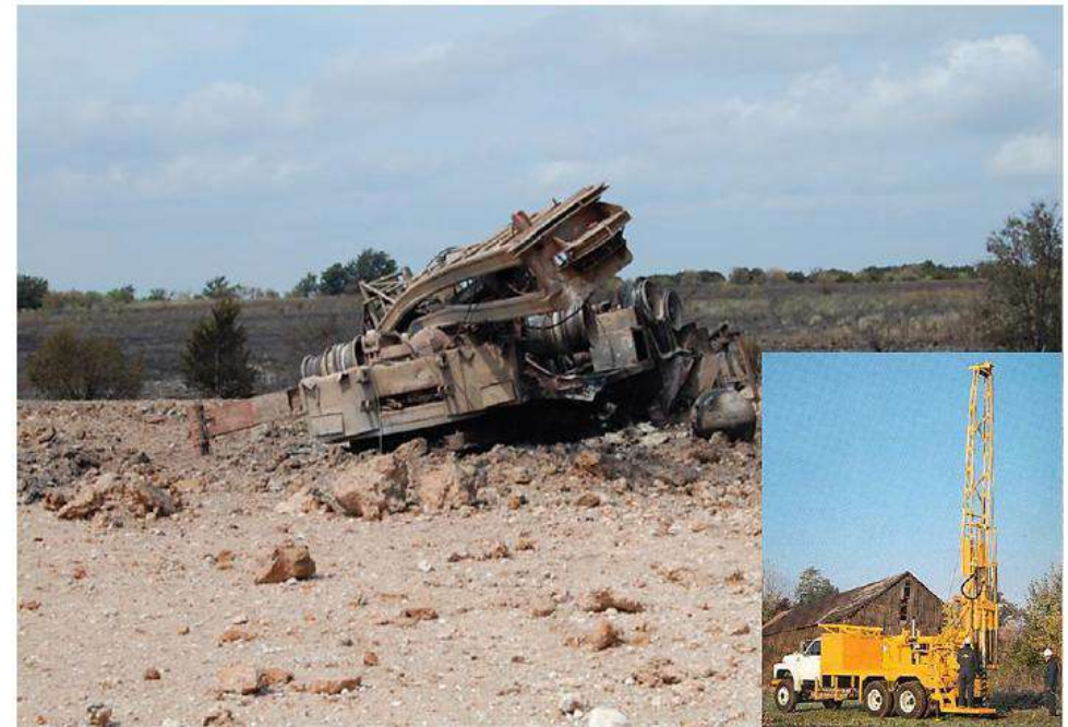
Figure 4. Upside-down, 60-ton C&H auger truck; exemplar truck shown in lower right
