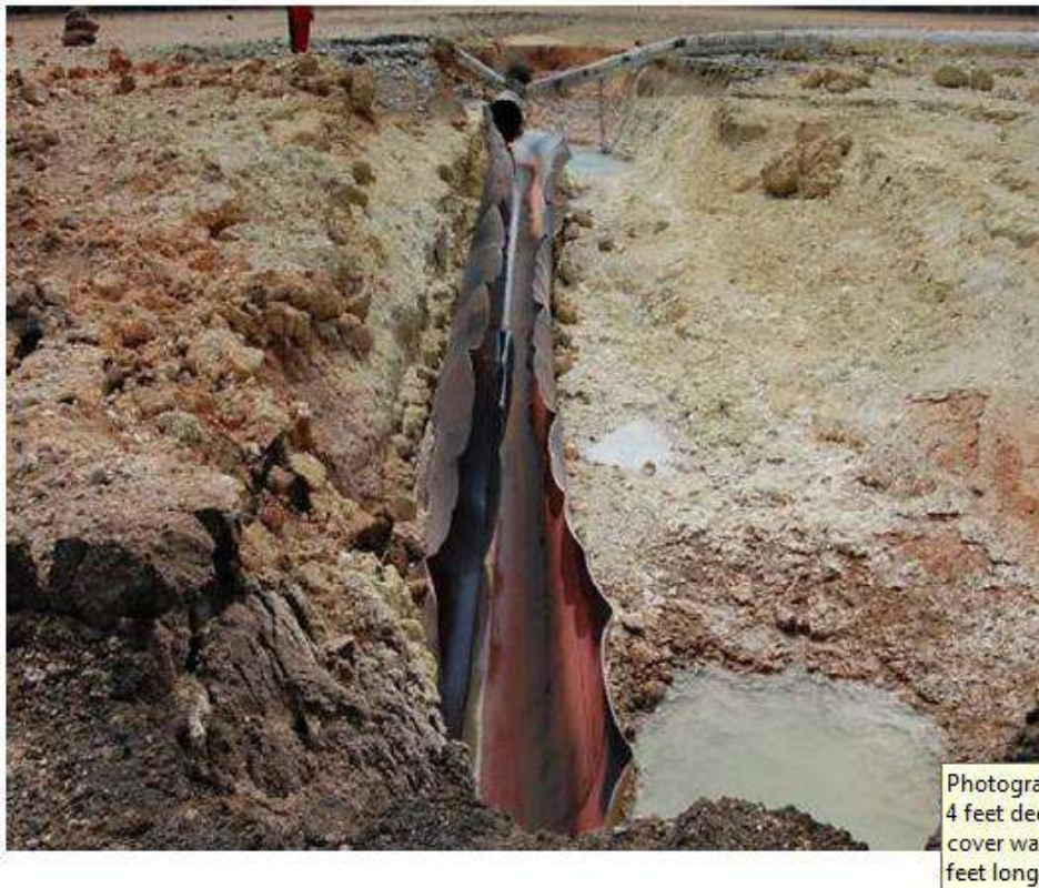
Figure 3. Ruptured section, about 110 feet long, of 36-inch-diameter Enterprise natural gas pipeline
